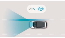
Lane Keeping Assist: The Lane Keeping Assist (LKA) uses the front multi-function camera to monitor the lines of the road. In case of an unintended lane departure, it warns you and can apply counter steering torgue to guide the car back to the lane.
