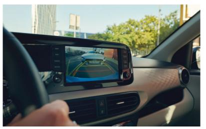
8" Multi-media display features Rear View Camera, dynamic AR guidelines and complete smartphone connectivity – available on SE Connect and above.
