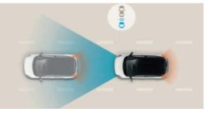
Forward Collision-Avoidance Assist (FCA): Sensing the road ahead with the multi-function camera, FCA warns you and then automatically brakes when it detects sudden braking by a car ahead. Includes pedestrian detection.
