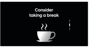
Driver Attention Warning (DAW): When a pattern of fatigue or distraction is identified, the system gets your atten-tion with an alert and pop-up message suggesting a break.
