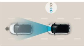
Leading Vehicle Departure Alert (LVDA): This clever feature for city driving alerts the driver when the vehicle in front departs from an idle state, like at a stoplight or in a traffic jam.
