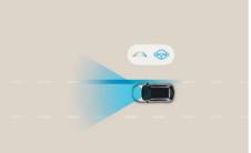
Lane Keep Assist (LKA): The Lane Keep Assist (LKA) uses the front multi-function camera to monitor the lines of the road. In case of an unintended lane departure, it warns you and can apply counter steering torque to guide the car back to the lane.
