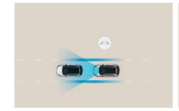
Lane Follow Assist (LFA): Smart sensors and the forward-facing camera detect when the car drifts from the centre of the lane, applying steering torque to hold road positioning for safety. The car also estimates the trajectory of the vehicle ahead and adjusts its position accordingly.
