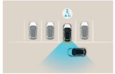
Rear Cross-traffic Collision Warning (RCCW): Sensors detect vehicles approaching from both sides when the New i30 is in reverse, avoiding collisions in congested or reduced visibility environments such as car parks.
