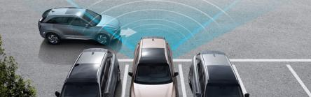
Rear Cross-Traffic Collision-Avoidance Assist (RCCA): Radar sensors in the rear bumper monitor cross traffic approaching from left and right side of the vehicle during reverse manoeuvers, and if necessary apply emergency braking to prevent collision.
