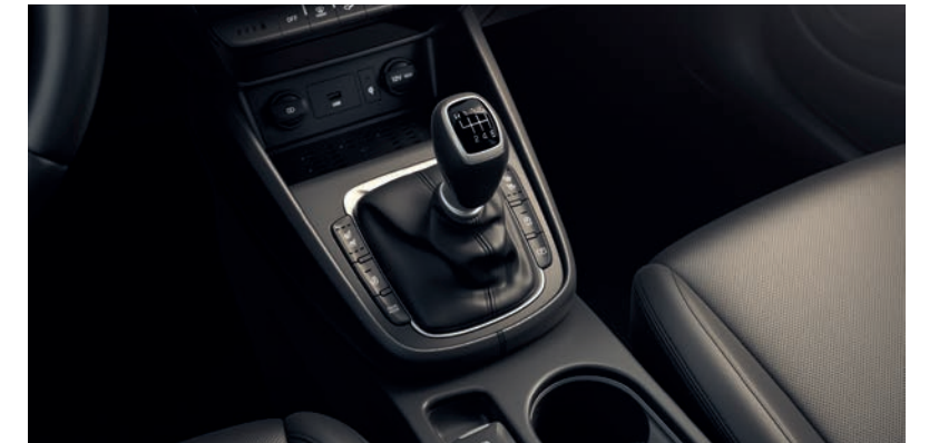
Six speed Intelligent Manual Transmission (iMT) standard on all 48V Mild Hybrid trims. Car shown is not to UK Specification.
