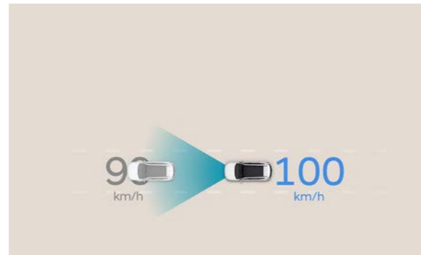
Smart Cruise Control (SCC): Automatically takes road features into account and adjusts your speed to maintain a safe distance from the vehicle in front.
