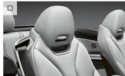
Exclusively available for BMW M4 Convertible Competition, the air collar releases pleasant, warm air around the head and shoulders, ensuring comfort when driving with the roof open.
