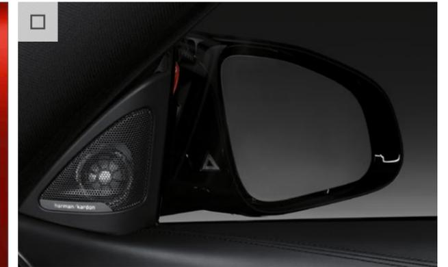
The harman/kardon loudspeaker system has a 600 watt digital amplifier, vehicle-specific equalising and loudspeakers with Chrome detailing.<sup>1</sup>
