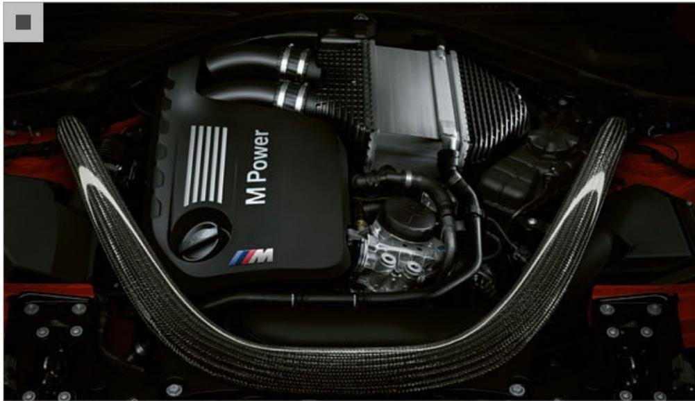
Made of carbon fibre reinforced plastic (CFRP), the precision strut brace increases frontend rigidity, steering precision and accuracy.
