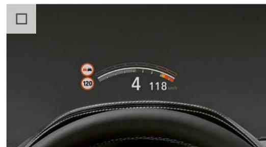
The full-colour BMW M Head-up Display with M-specific functions projects all relevant journey information directly into the driver's field of vision. With the press of a button, the driver can switch to the M-specific display, which includes a gear indicator, the rpm as a dynamic range curve and shift lights indicating the optimal moment to shift gear. Image may show additional optional equipment.
